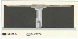
Gripnails and Insul-Tacks have tapered and tempered steel points which close to form a ball and socket arrangement within the thickness of the sheet metal.
