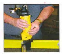
**Standard Compression Riveters** may be adapted for applying fasteners to extrusions or tubing.
