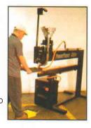
The quality of a welded fastening is a combination of fasteners and equipment. For this reason, we manufacture a complete line of equipment which matches the requirements of our weld pins. Floor model machinery applies fasteners with the touch of a foot pedal.
