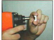
Tack-Mounts are securely held on to the tip of the air tool with a magnetic driver.
