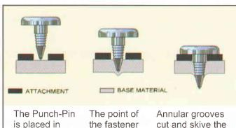
the fastener cut and skive the the hole of the pierces the metal for a permanent fastening. attachment. sheet metal.
