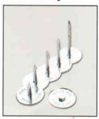
PowerPoint weld pins have a cupped head which prevents damage to insulation and a pyramid shaped point for a positive electrical contact. Several sizes are available to fasten insulation from 1/4 inch to 2 inches.
