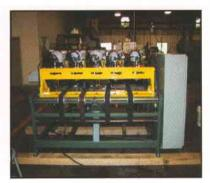
**Integrated Multi-fastener automation** may be used to apply up to 300 fasteners per minute.
